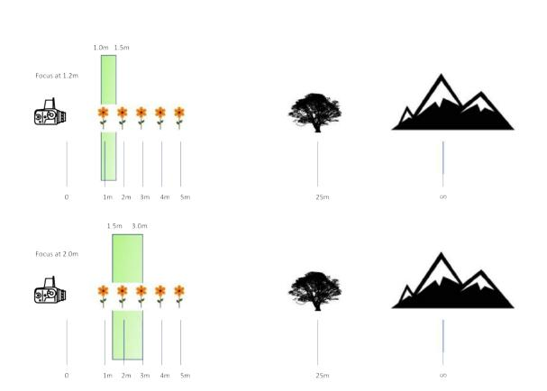
The green-shaded area in these pictograms represents the calculated depth of field when using a camera having an APS-C sensor with a 30 mm focal length lens, set to f8.
